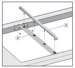
Fit the cover strip ④ into the holes in the spacer bar ②.
